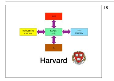
"The Harvard architecture is a <u>computer architecture</u> with physically separate <u>storage</u> and signal pathways for instructions and data."
